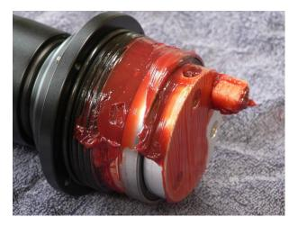
**o.** Review the greased components and compare the amount of grease with the photographs; generous greasing is required to maximize lubrication of the Thrust bearing and protect against corrosion. If any bare metal is exposed, apply a light coating of grease until all surfaces are protected.
