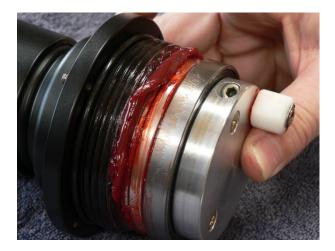
i. Completely fill the volume between the preload bearing and the start of the thread with grease.
